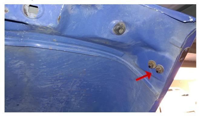
9. Installation complete. Check latch for proper movement and check that the latch closes snuggly.
