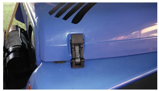
2. Starting with the lower portion of the latch located on the front fender remove the factory 15mm nut
