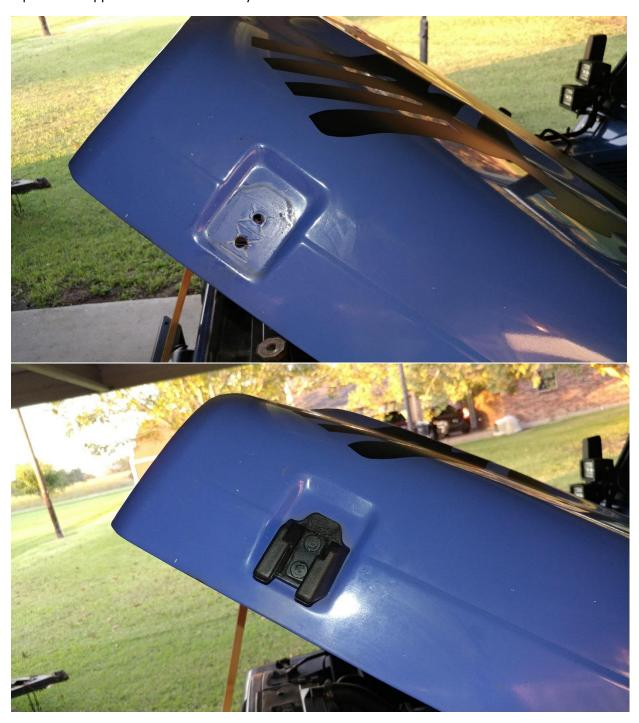
7. The factory nuts are a washer/nut combination, I choose to reuse the factory hardware
