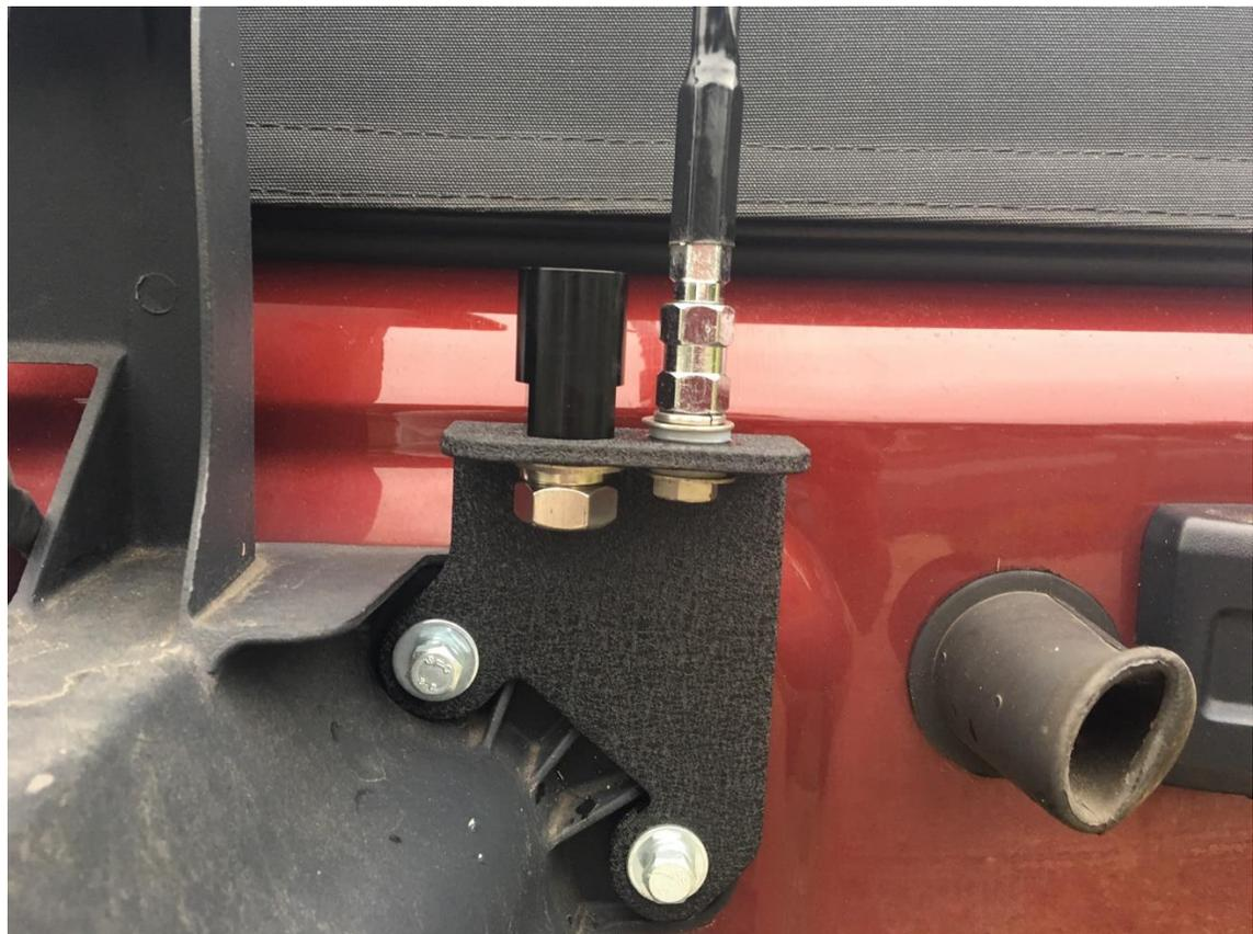
6. Attach the whip to the whip mounting cylinder.
