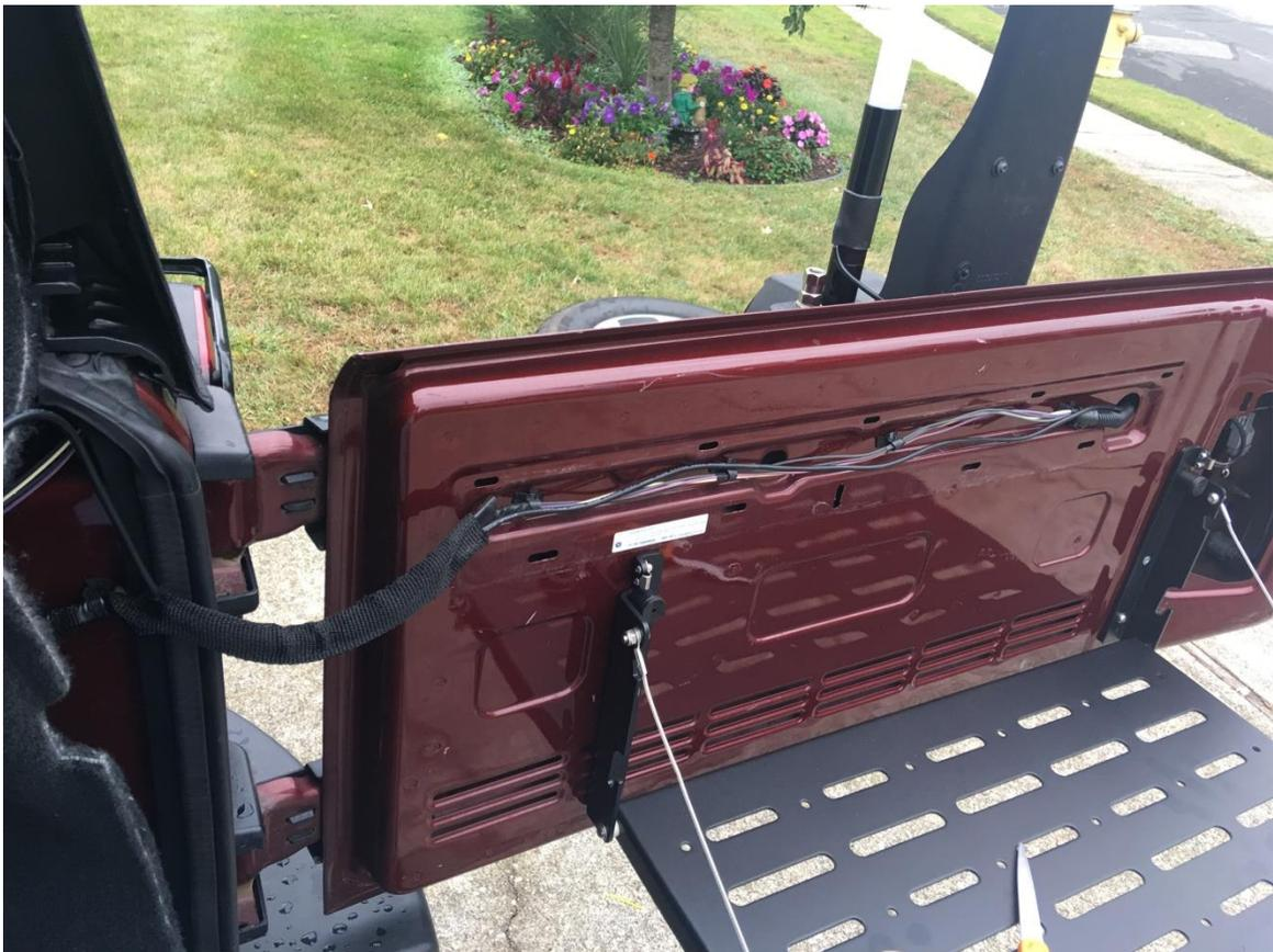
10. At this point, you will need to find a place to splice the whip wire into. I chose to splice it into some lights that I have that are underneath the seats, but it will vary from person to person.
