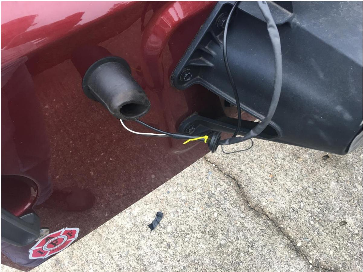
9. Run the wire through the area that the third brake light wiring is held.
