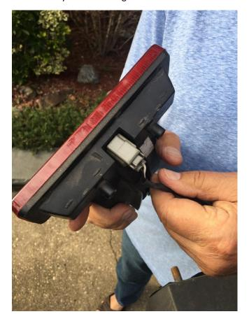
4. Reinstall the wiring harness on the Recon Third Brake light
