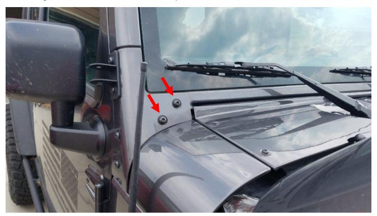
**3.** Using the supplied bolts and washers, install the brackets. The OCF logo should be facing outward. Make sure to place the supplied gasket between the bracket and your paint. Tighten the bolts using a 5mm allen wrench.
