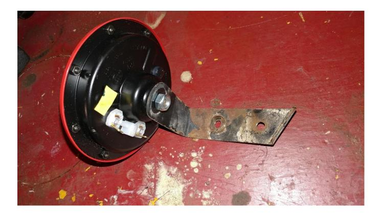
8. Reinstall the factory brackets with the new Hella Twin Supertone Horns attached using the factory 13mm bolts
