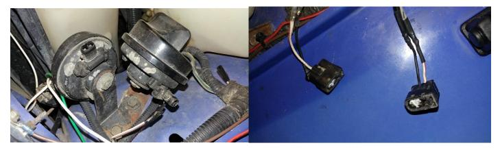
3. Remove the two 13 mm bolts holding the factory horn brackets in place
