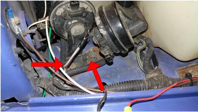
4. Remove the 13 mm nut holding the factory horns to the factory brackets
