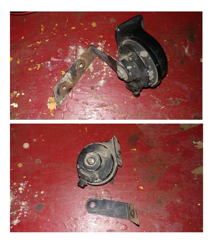
5. The Hella Twin Supertone Horn Kit provides metal mounting tabs. I choose to use the factory mounting brackets for ease of installation.
