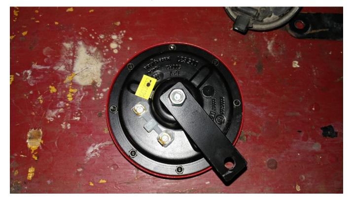
6. Remove the 13mm nut on the Hella Twin Supertone Horn
