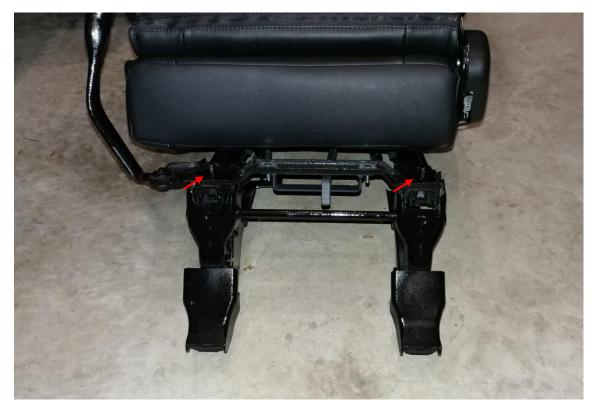
10. Attach the Corbeau slider arm to the factory slider arm, using the provided 10 mm bolt and nut
