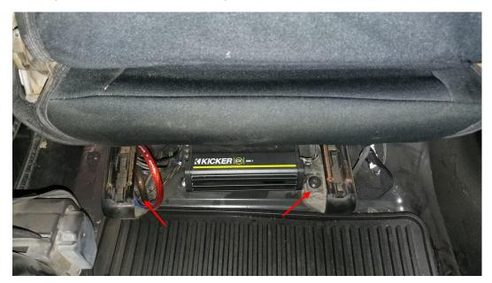
3. When removing the seat from the Jeep be very careful and unplug the seat belt light harness connector. Located on the side closest to the center console
