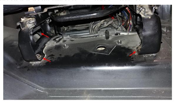
10. Driver side install complete. Pull and shake seat to check for any loose bolts. Check the factory slide function.
