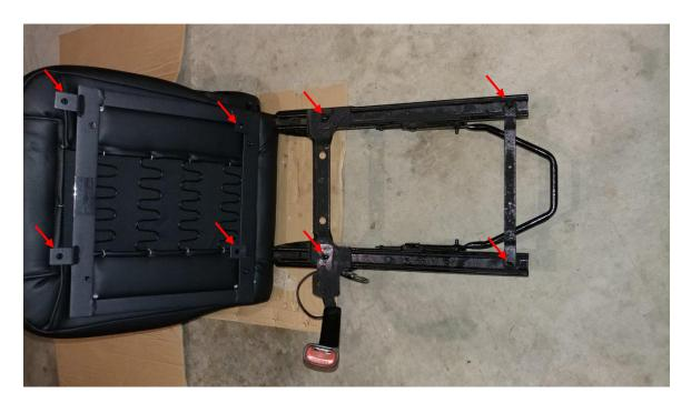
8. Reinstall the 4-13 mm factory nuts onto the factory assembly studs. This will be a very tight fit, a 13 mm open end wrench/Box end wrench will be required.
