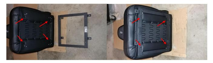
7. Place the Driver's side seat with seat bracket adapter attached on to the factory seat assembly studs. Line up the front and rear before applying pressure.
