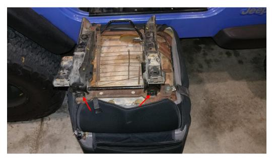
6. Remove the 4-13 mm nuts from the factory seat slider studs. May require a  $\frac{1}{4}$ " drive shallow socket, it is a tight fit.
