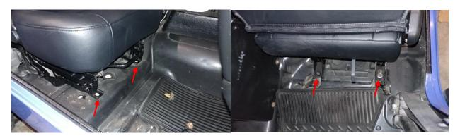
13. Passenger side install complete. Pull and shake seat to check for any loose bolts. Check factory "fold and tumble" function.
