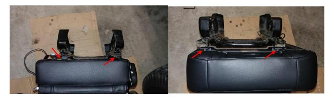
9. To reinstall the new seat into the Jeep, first reconnect the seat belt light harness connector. Located on the side closest to the center console. Second secure the 3 – 13 mm bolts and 1 – T50 Star Bolt
