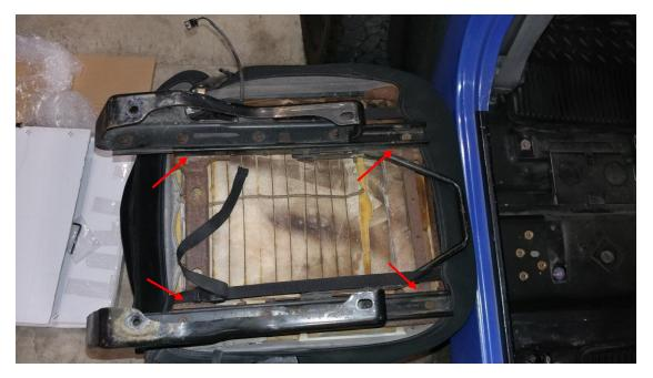
5. Remove the 4-13 mm nuts from the factory seat slider studs. May require a  $\frac{1}{4}$ " drive shallow socket, it is a tight fit.
