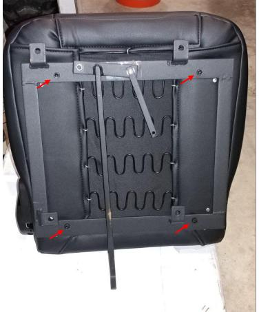
8. Install the Corbeau slider handle limiter with the provided 2 – 10 mm bolts into the factory holes
