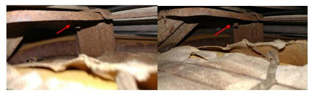
6. Attach the Corbeau Seat Bracket Driver Side - D1120NS to the Corbeau Moab Seat bottom with the provided Allen screws (provided with seats) and provided 9mm Allen wrench (provided with seat brackets)
