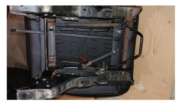
11. Reinstall the 4-13 mm factory nuts onto the factory "fold and tumble" assembly studs. This will be a very tight fit, a 13 mm open end wrench/Box end wrench will be required.
