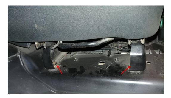
2. Using the slider push the Driver's seat all the way forward. Remove the 1-13 mm bolt and 1-T50 Star Bolt
