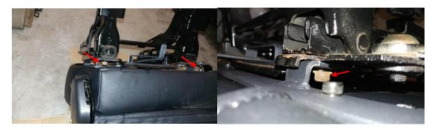
12. Reinstall the new seat with the factory "fold and tumble" assembly attached into the Jeep. Secure the 3-13 mm bolts and 1-T50 Star Bolt
