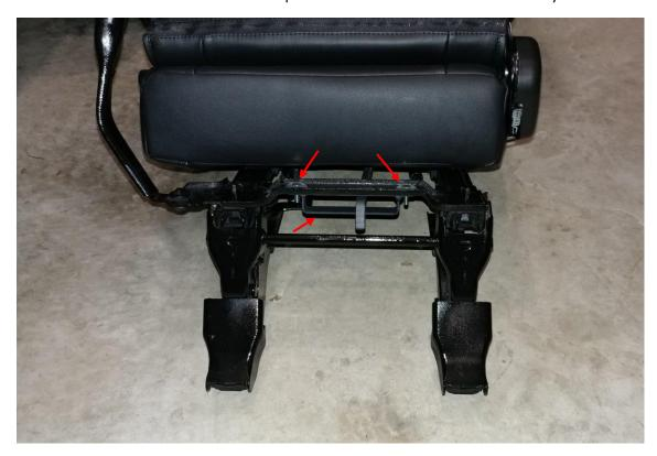
9. Place the passenger side seat with seat bracket adapter attached on to the factory seat "Fold and Tumble" assembly studs. Line up the front and rear before applying pressure.
