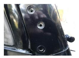
11. While a second person holds the opposite side, Using  $5/16'' \times 1 \frac{1}{2}''$  bolts with serviceable thread locker applied, and 5/16'' washers, mount the light bar and snug up the bolts. Make sure the mount does not interfere door opening / closing. Repeat for the other side,
