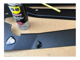
3. Make sure grommet is fully inserted with the large side facing to the outside.
