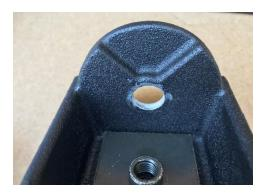
5. Assemble the Rota Hood Casting, Rota Square Casting and the Welded Nut using the 3/8" bolt. Tighten fully, then loosen by a ½ to 1 full turn. This will be fully tightened later. Repeat for other side.
