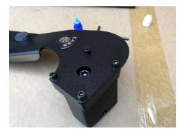
8. Insert the Cross Bar into the Rota Hood Casting. Secure using a 5/16" bolt inserted from the top and the double hole washer and nylon locking nut. Repeat for the other side. The bar is complete and ready to mount.
