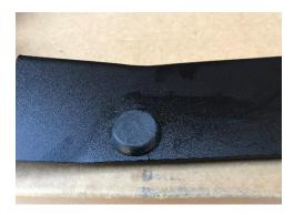
4. Using a rotary tool, clear the power coat paint from the inside of the Rota Hood Casting. The welded nut MUST fit inside the Rota Hood Casting sitting flush.
