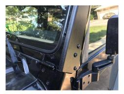
12. With the light bar mounting complete, Level the bar rotation to the desired angle and secure the 3/8" bolt on both ends of the light bar.
