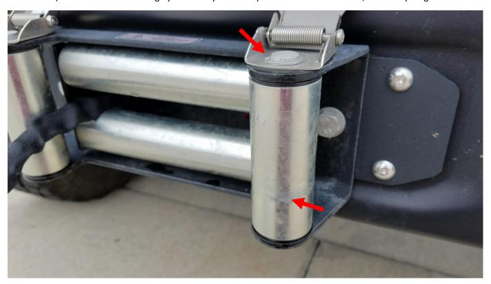
**5.** Then feed in your new synthetic winch rope through the fairlead and around the bottom side of the drum as shown below. Use the bolt removed in step 3 to attach your new rope as shown below.
