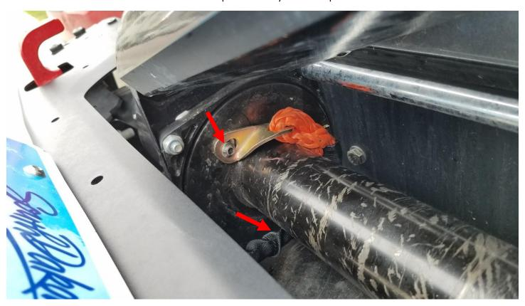
**6.** Next, crank up your Jeep, connect your winch remote and re-engage the winch clutch. Using gloves to hold the rope tight, begin to wind the rope in. *Caution:* Be very careful not to get your hand too close to the fairlead while winching. Your hand could get caught and severely injured.
