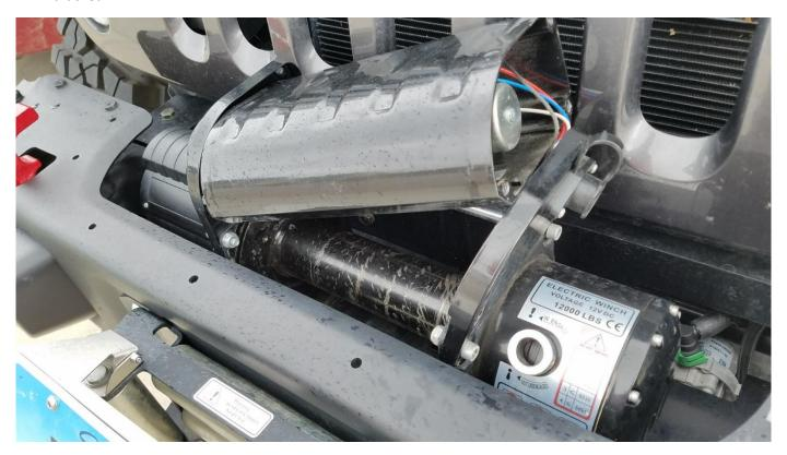
**3.** At the very end of the cable there will be a bolt holding your cable to the drum. Use a 5mm Allen wrench to unscrew and remove this bolt.
