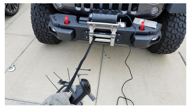
7. Wind in the rope initially until you have 1 complete wrap all the way down the drum as shown below.
