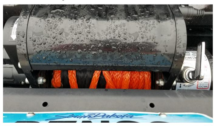
**10.** When you get to the last few feet of rope, stop winching. Attach your hook to the end of the rope as shown below, and hook it to your desired location. Then finish winching in the rope until it's tight enough not to bounce around.
