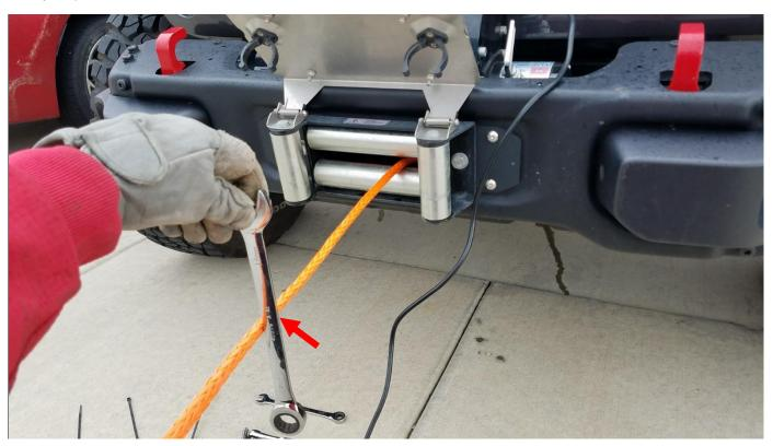
**9. My recommendation-** Option 2: No weight required, just pull the rope tight. After step 7 feed the rope side to side in a criss cross pattern. The rope will come out looking messy as shown below, but it is far less likely to "submarine" while winching.
