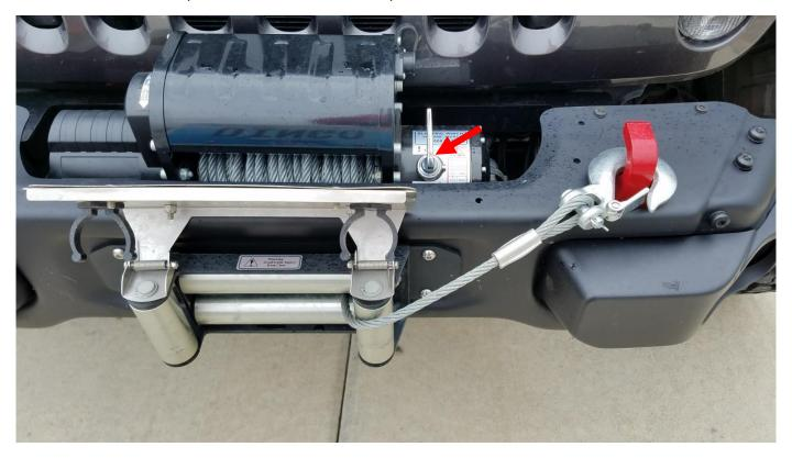
2. You may need extra room to work with, so I recommend you partially or fully remove your winch solenoid. For my winch that required 5mm, and 6mm Allen wrenches to remove the bolts on both sides of the solenoid box. Note: For many other winches (Including Barricade), you simply need a screwdriver to loosen the solenoid mount bracket.
