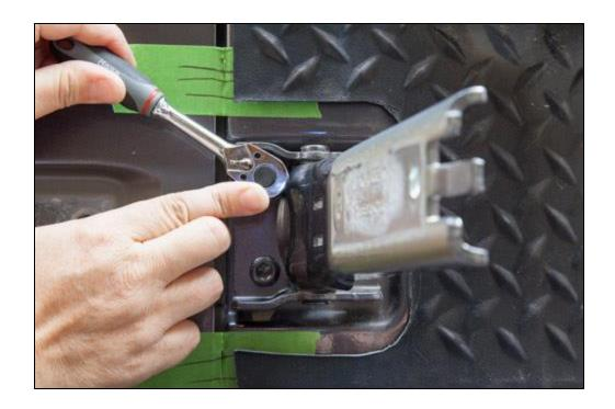
13. There are two spare tire bump stops on the tailgate. Remove the one closest to the hinge by grasping firmly and pulling.
