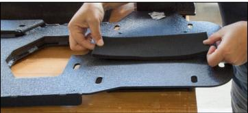
16. Position the Barricade Tire Carrier Bracket Mount ears in the hinge mounts.
