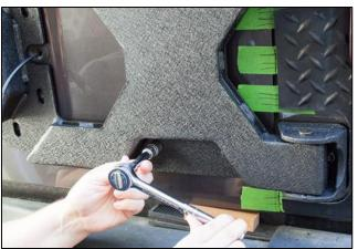
19. Use the eight factory bolts (removed in Step 5) to secure the 4 corners of the Tire Carrier Bracket Mount. Check the lines on the painter's tape to ensure the tailgate hasn't shifted. If required, adjust the height of the tailgate using the shim. When properly aligned, tighten all eight bolts using a 13mm socket and wrench. A short socket extension bar may make the job easier.
