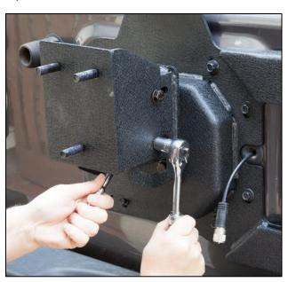
27. Loosely secure the supplied upper and lower 3<sup>rd</sup> tail light brackets together using the provided Allen bolts, washers, lock nuts, and a #4 Allen wrench.
