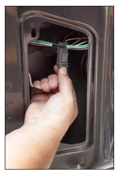
4. On the exterior of the tailgate, continue removing the 3<sup>rd</sup> brake light cable. Squeeze the rubber grommet with your fingers and separate it from the tailgate. Pull the 3<sup>rd</sup> brake light cord and connector free of the tailgate.
