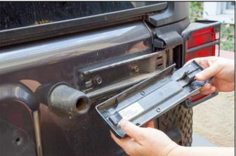
8. Remove the body hinge mount covers. Grasp the plastic hinge mount cover from the side closest to the tailgate and rotate out / pull gently to remove. Repeat to remove second hinge mount cover.
