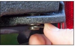
18. Position the thinnest spacer behind the top of the Tire Carrier Bracket Mount before threading the supplied 13mm bolt with washers through it. Repeat with the lower part of the Mount, using the thickest spacer. Tighten all 4 bolts with a 13mm socket & wrench.
