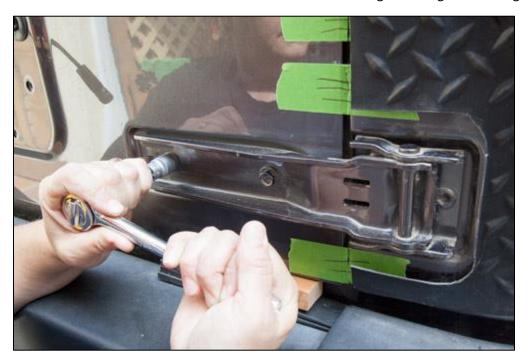
12. Gently pull the hinge to the open position. Using a T50 TORX bit, remove the three TORX bolts holding each hinge mount to the body of the Jeep. Save these bolts as you will re-use them in Step 14.
