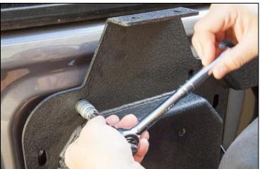
20. Loosely bolt the Tire Carrier Base to the Tire Carrier Bracket Mount using the four supplied 18mm bolts and washers. Secure, but do not tighten. You will need to dry fit the tire to determine the proper height.
