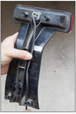
30. Position the Barricade brake light bracket on the backside of the factory 3<sup>rd</sup> brake light. Make sure the brake light wiring isn't being pinched between the two parts.
