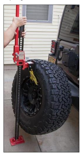
25. Remove the spare tire. Position and tighten the Tire Carrier Bracket Base to the Tire Carrier Bracket Mount with an 18mm socket & socket wrench. An extension bar may make the job easier.
