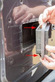
7. Remove the tailgate hinge covers. Grasp the plastic hinge cover and pull gently to remove the tailgate hinge cover. Repeat to remove the second tailgate hinge cover.
