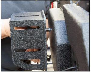
21. Loosely bolt the Spare Tire Carrier to the Tire Carrier Base with the supplied bolts, washers and nuts.
