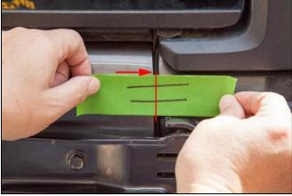
10. Shim the bottom of the tailgate at both the hinge and handle sides.
