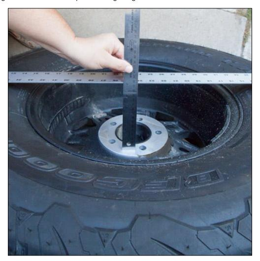
23. Place the straight edge on top of the loosely installed Spare Tire Carrier. Use a ruler to measure to the Tire Carrier Mounting Bracket. Position the Tire Carrier to the correct backspacing. Do not tighten all the way, but secure the Tire Carrier with a 5/8" socket on the bolt head and a 17mm socket on the nut, making certain that all parts are plumb and level.
