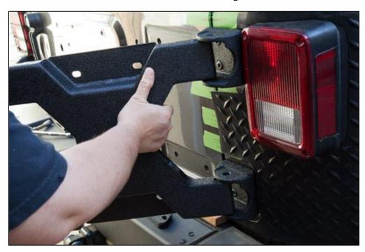
17. Slide the pins into the hinge mounts and Tire Carrier Bracket Mount. You may need to use a rubber mallet to fully seat the hinge pins. Secure the bottom of each hinge pin with one of the provided C-clips.
