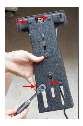
32. Loosely mount the spare tire on the tire carrier using a 19mm socket and tire iron. A farm jack may make lifting the spare tire easier.
