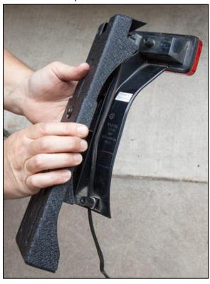
31. Secure the bracket to the brake light using the four factory TORX screws removed in Step 28, a T20 TORX bit, and wrench.
