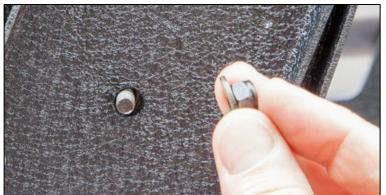
28. Disassemble the factory 3<sup>rd</sup> brake light bracket by removing the four TORX screws from the rear of the factory tire carrier. Use a T20 TORX bit and socket wrench. Save the TORX screws as you will re-use them in Step 32.
