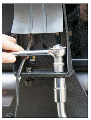
35. Reinsert the factory 3<sup>rd</sup> brake light wiring into the tailgate by feeding the connector and wiring through the tailgate hole. Secure the wiring with the rubber grommet.
