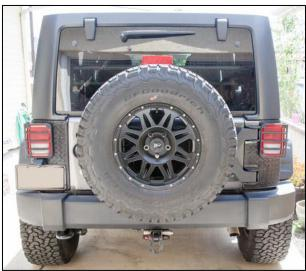
2. Remove spare tire with a tire iron and socket that fits your lug nuts (typically 19mm).
