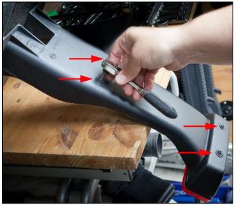
29. Slide the 3<sup>rd</sup> tail light wiring out from under the factory bracket tabs and route it to the right of the channel.
