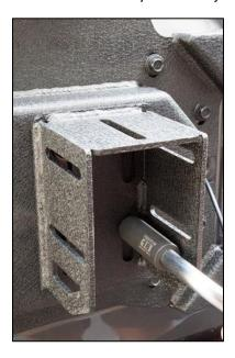
26. Tighten the Tire Carrier to the Tire Carrier Base with a 5/8" socket on the bolt head and a 17mm socket on the nut, making certain that it's plumb and level.
