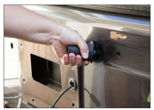
14. Install the new hinge brackets using the six factory T50 TORX bolts that were removed in Step 12 (three bolts per hinge mount). Tighten them with a wrench and T50 TORX bit; they will self-center when secured.
