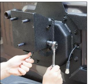
24. Dry fit the spare tire to verify the placement of the Tire Carrier Base (height) and the Tire Carrier (depth). Adjust the Tire Carrier Base and Tire Carrier as needed to ensure the spare tire is positioned close to the tailgate and bumper. A farm jack may make dry fitting the tire easier.
