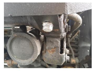
9. Install remaining bolts into upper mounting points, leave loose until all bolts have been threaded. After all bolts have been threaded, tighten all six bolts.
