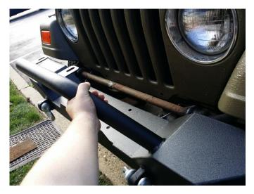
7. Stack washers onto bolts with the lock washer going on first.
