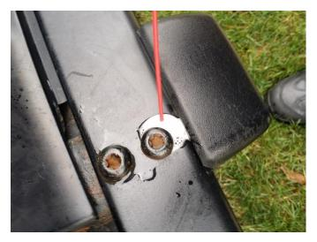
2. Using the T-55 torx bit, remove the four upper bolts.
