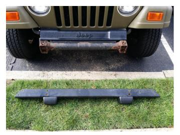
5. Using a 10mm socket, remove bolts on sides of sway bar cover and remove cover.
