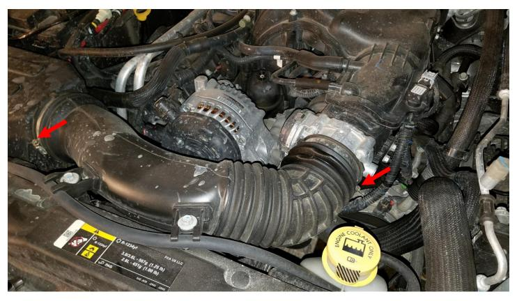
2. Using a 10mm socket, remove the 2 bolts on the front of the intake tube.
