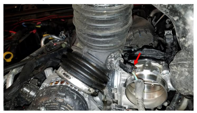
8. Reinstall the intake tube and use a 10mm socket to tighten the front 2 bolts.
