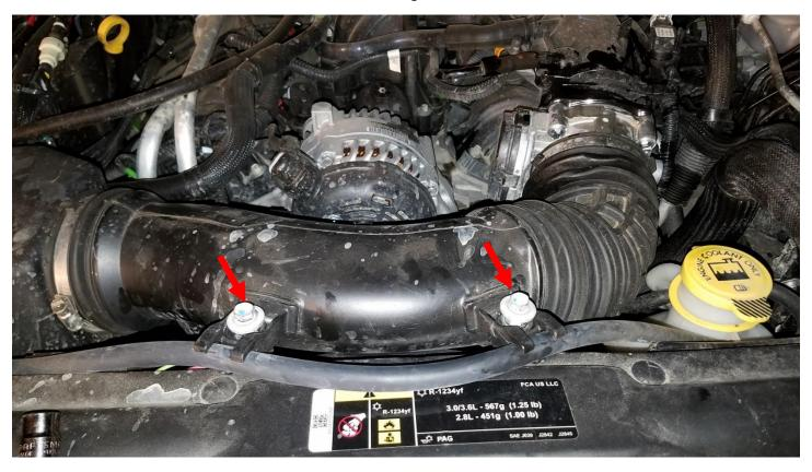
**9.** Make sure both ends of the intake tube are fully seated on the throttle body and the air box, then tighten the clamps using an 8mm socket. Be careful not to overtighten the clamps.
