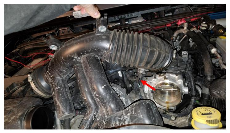
**4.** Using an 8mm socket and socket extension, remove the 4 bolts holding on the throttle body.
