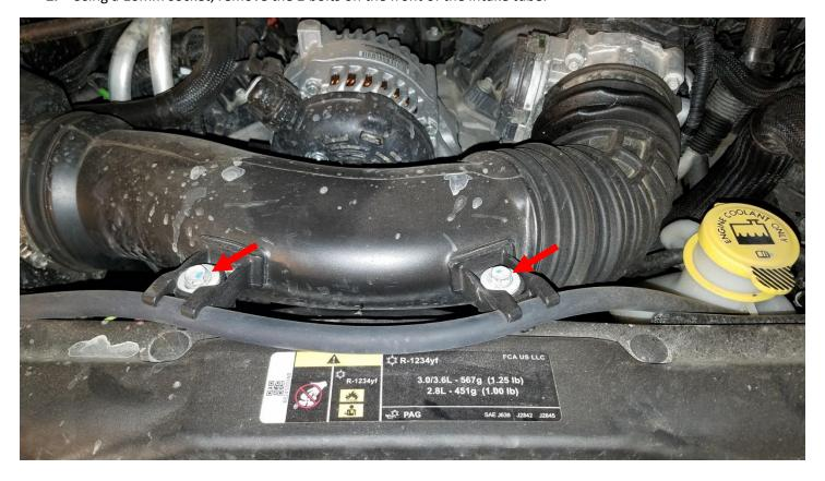
**3.** Lift up the intake tube, and use needle nose pliers to unclip and remove the temperature sensor from the underside of the intake tube. Then place the intake tube to the side out of the way.
